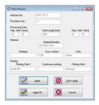
If activated (chapter 7.1) the preview dialog shows up for every wire converted. It's primary use is for error hunting when the results of conversion are undesirable.
